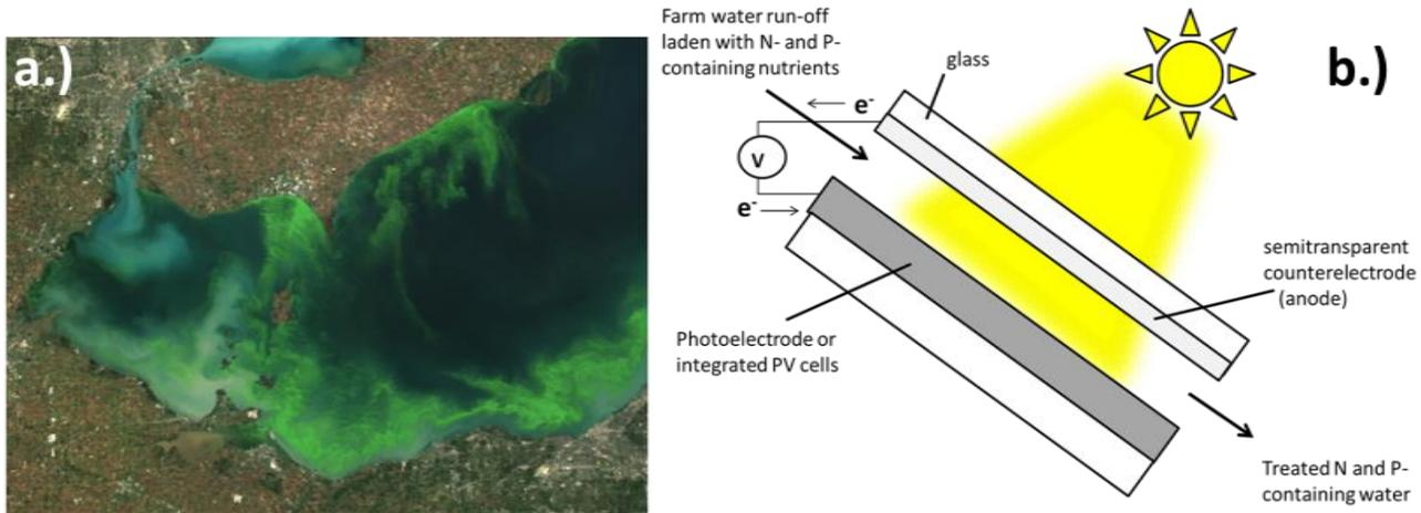
**Figure:** a.) Algae blooms in Lake Erie (AP Photo courtesy of NOAA). b.) Solar reactor for treatment of nutrient-laden water that has run-off from fields.
