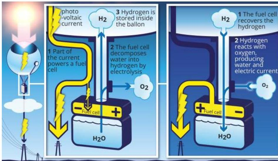
**Figure:** Schematic describing the basic idea of a solar-hydrogen high altitude balloon.[1]
