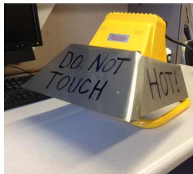
**Figure 3.** Work lamp with metal shield constructed such that bright light does not shine into the audience's faces and cause a safety hazard.
