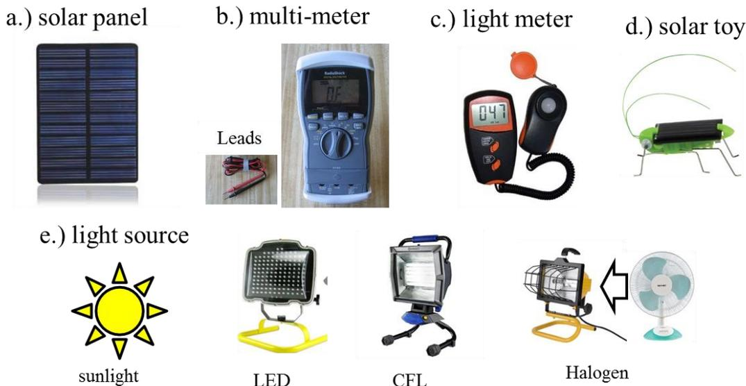
**Figure 2.** Key supplies used in the outreach activity. There are several light source options as described in the text. Use of a high power halogen work lamp is discouraged, but can be used with caution and under direct supervision.
